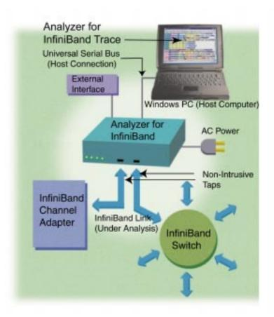
The Analyzer for InfiniBand provides on-the-fly detection of and triggering on such events as Packet Headers and Errors. Whether recording manually or with a specified trigger condition, the Analyzer for InfiniBand continuously records the link data in a wrap-around fashion until manually stopped or until the trigger event is detected and a specified post-trigger amount of link data is recorded.
